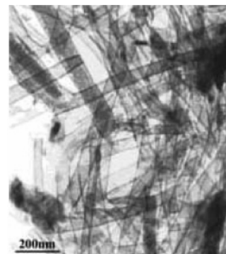
Figure 18. SnS 2 nanotubes sample synthesized with hydrothermal method. Reprinted with permission from ref 169 (Figure 3c). Copyright 2003 Springer.
